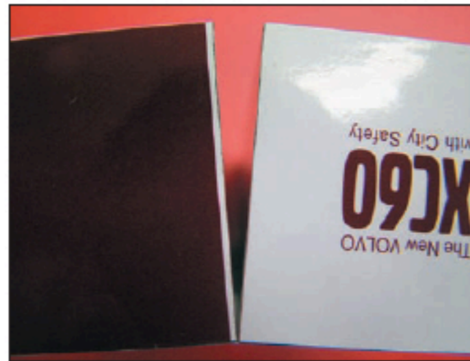
Placing different visuals alongside the die-cut may result in "bleeding"
